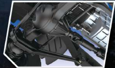
Rear suspension: 4-linkage suspension w/damper cylinder
