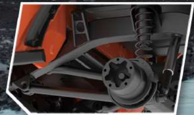
Rear suspension: 4-linkage suspension w/damper cylinder
