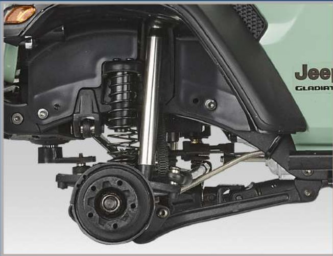
Front Suspension: 3-linkage suspension w/coil springs
